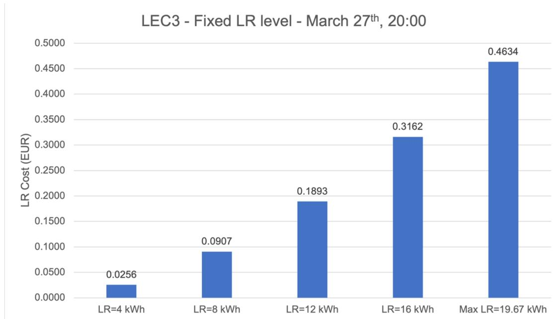
Figure 35: Cost of load reduction for different requested LR levels on March 27<sup>th</sup>, 20:00.
