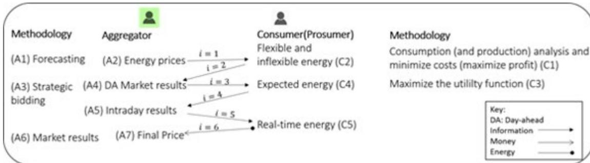
Figure 10: Interactions between the LEC aggregator and its members, and their methodologies.
