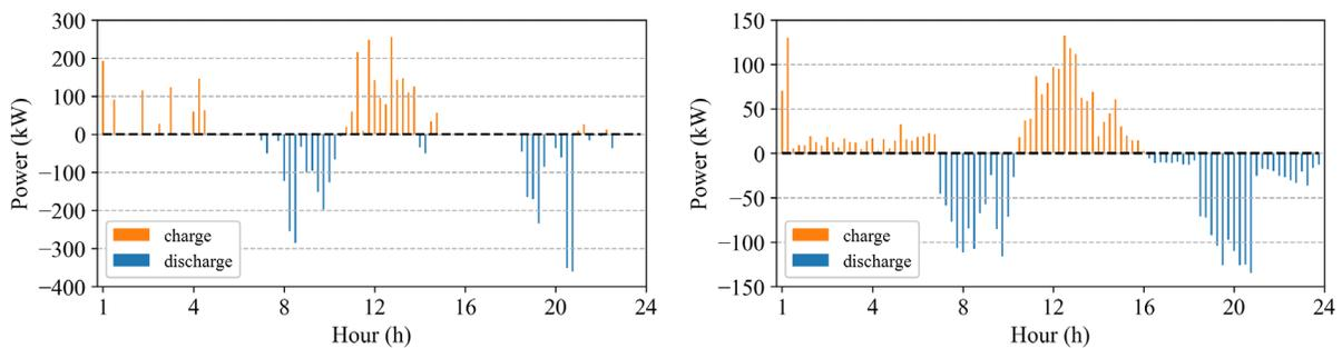
Figure 65: Storage charging and discharging power for Optimization and RL approaches.
