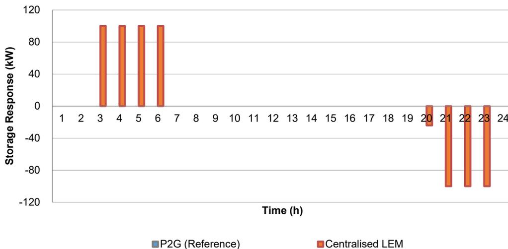
Figure 58: Aggregate charging / discharging power of ESs for two scenarios.
