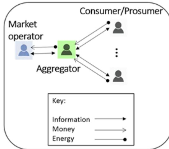
Figure 8: Communication protocol between players and the different interactions between the aggregator and the market operator.
