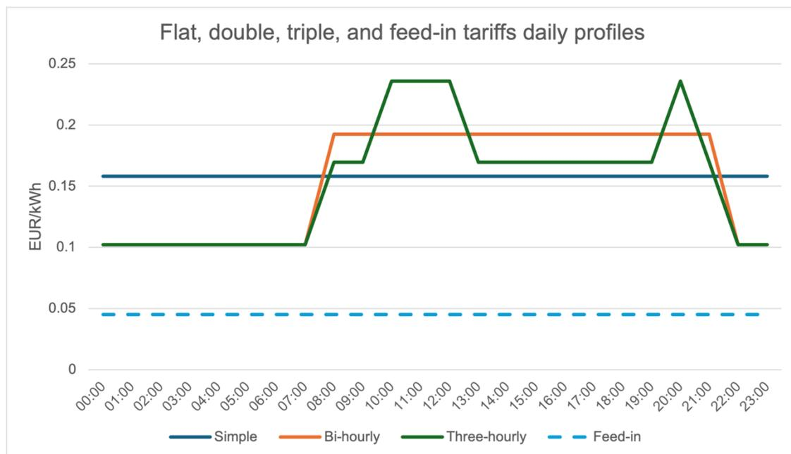
Figure 17: Flat, double, triple, and feed-in tariffs daily profiles.
