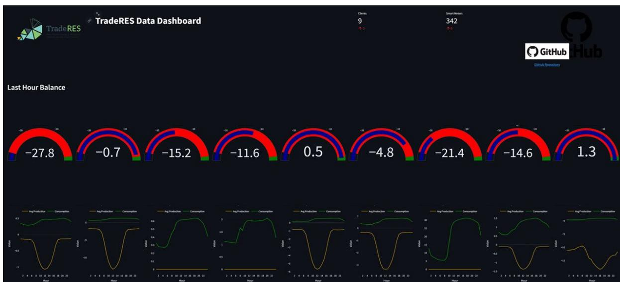
Figure 12: Screenshot of the blockchain based energy data dashboard, showing both last hours balance, and the consumption and production over the last day
