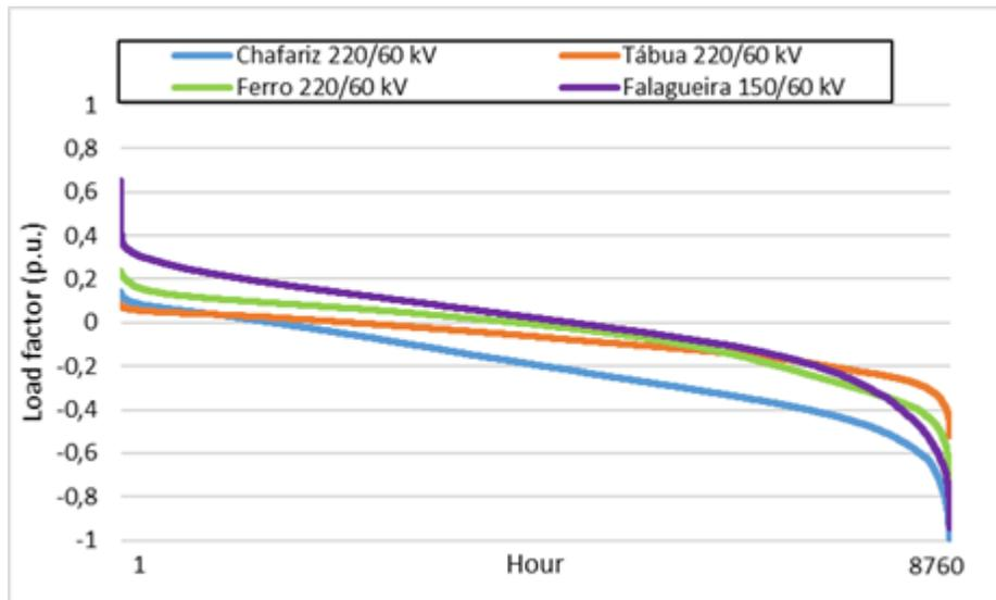
Figure 42: Substations load factors using the projected 745 MW PV and LEC flexibility in 2018.
