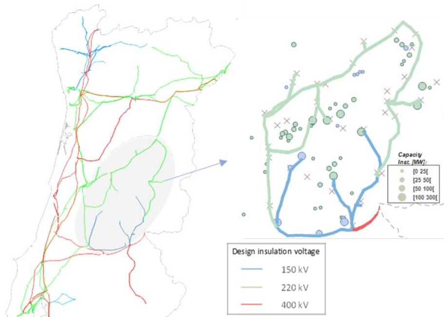
Figure 19: Location and capacity of the transmission lines, the distribution substations where consumers are connected to (crosses), the hydro (blue circles) and wind power plants (green circles) before investing in solar PV.
