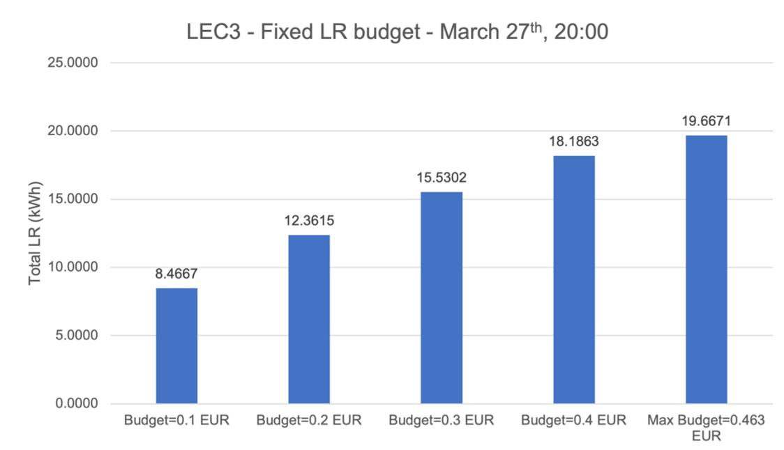
Figure 39: Cost of load reduction for different LR budget on March 27<sup>th</sup>, 20:00.
