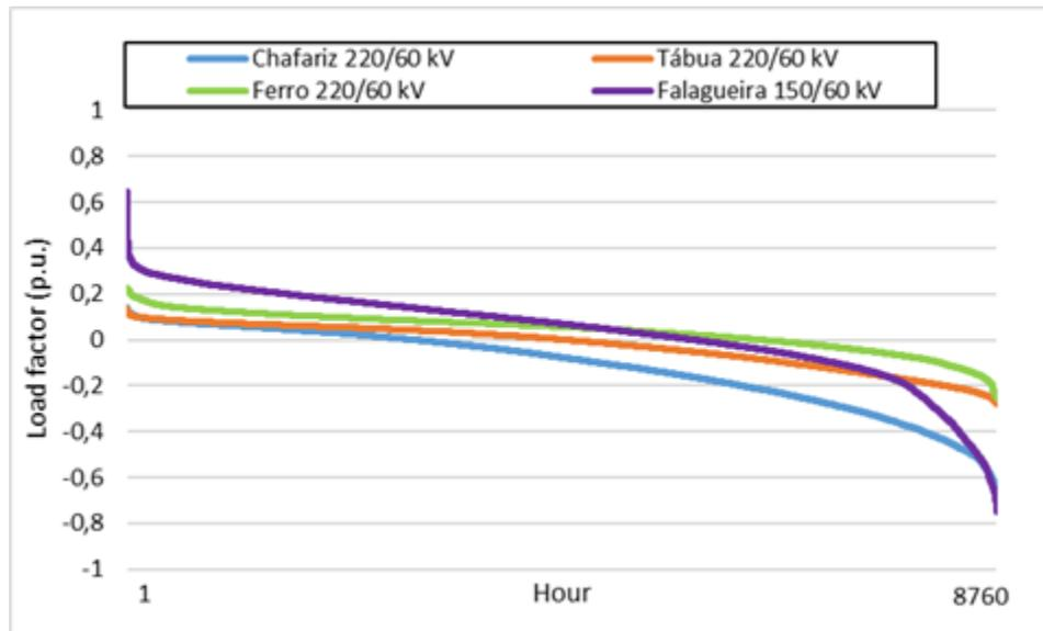
Figure 40: Load factors during 2018 of the most loaded substations. A positive load factor means the energy flow goes from the transmission to the distribution grids.
