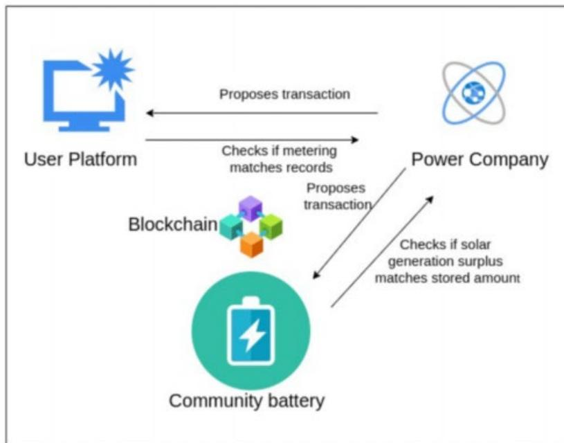
Figure 11: Visualisation of how the blockchain-based energy trading platform is set up
