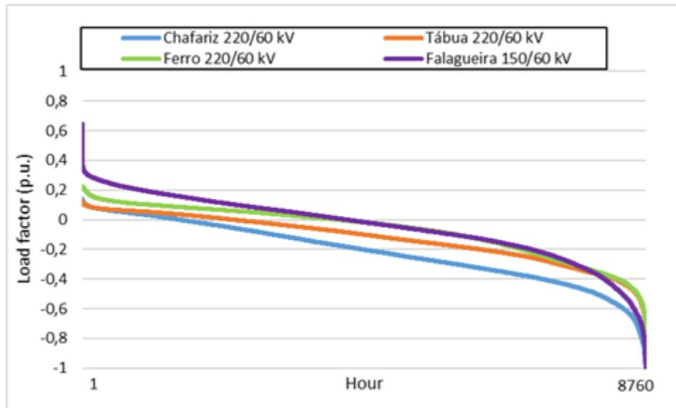
Figure 41: Substations load factors during 2018 using the new projected 745 MW of solar PV.
