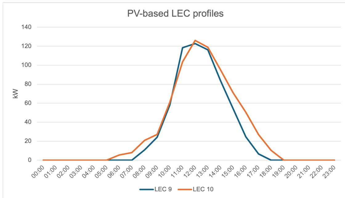
Figure 18: PV-based LEC generation profiles.
