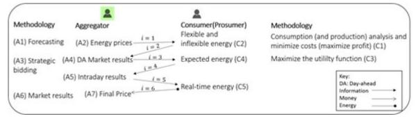
Figure 10: Interactions between the LEC aggregator and its members, and their methodologies.
