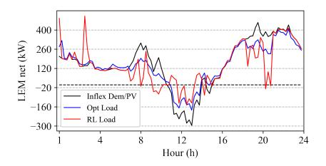
Figure 69: Community aggregate net profiles of 250 households for Optimization and RL approaches under Double-auction scheme.
