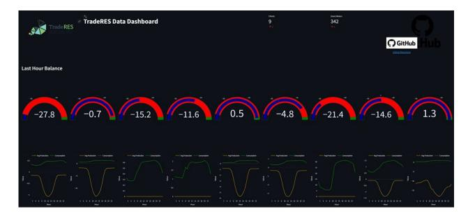
Figure 12: Screenshot of the blockchain based energy data dashboard, showing both last hours balance, and the consumption and production over the last day
