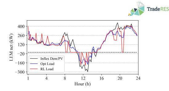
Figure 66: Community aggregate net profiles of 250 households for Optimization and RL approaches under Mid-market rate scheme.
