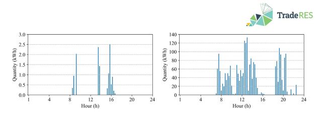
Figure 68: Local trading quantity for Optimization and RL approaches under Double-auction scheme
