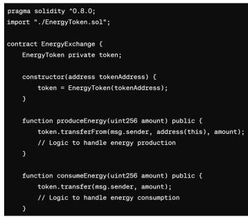
Figure 14: Code for the EnergyExchange Contract
