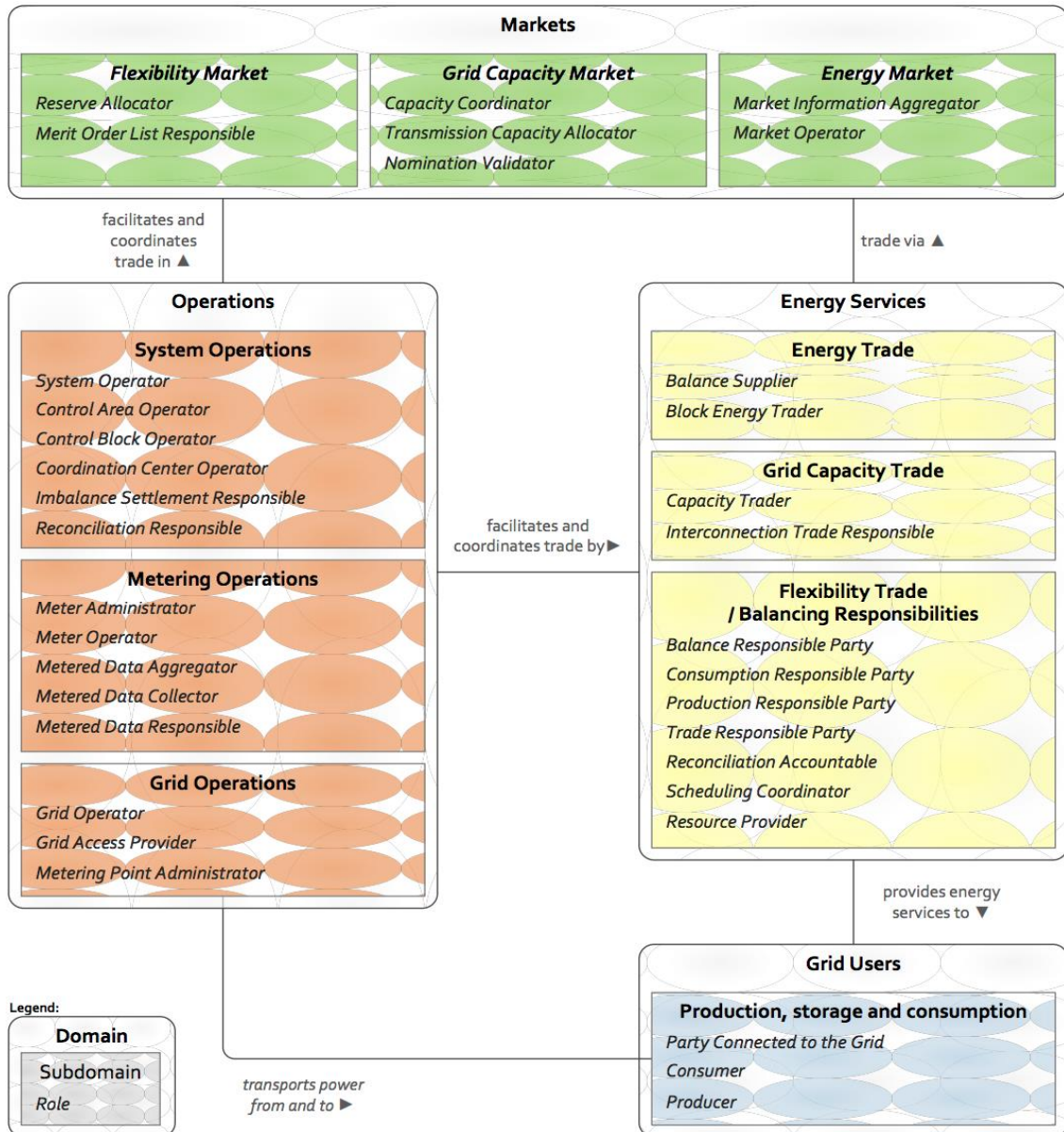
Figure 8: The HEMRM roles included in the European Conceptual Model for the Smart Grid.
