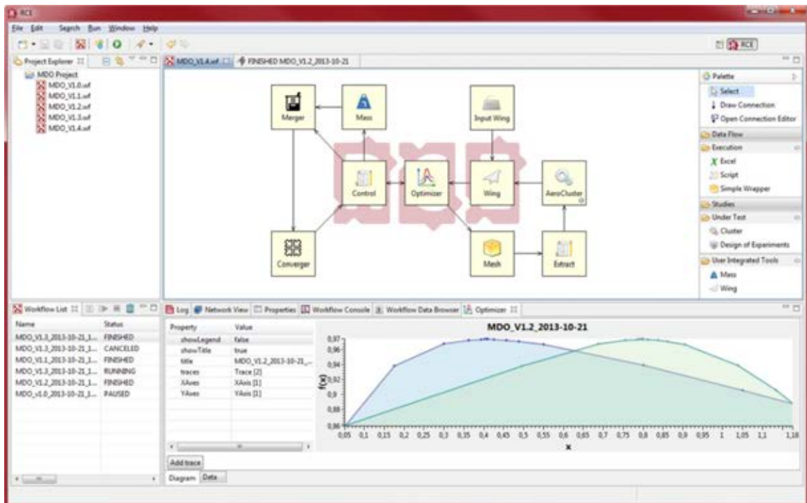
Figure 2. RCE's graphical user interface: Workbench with different views and opened workflow editor, taken from (RCE-10 User Guide)
